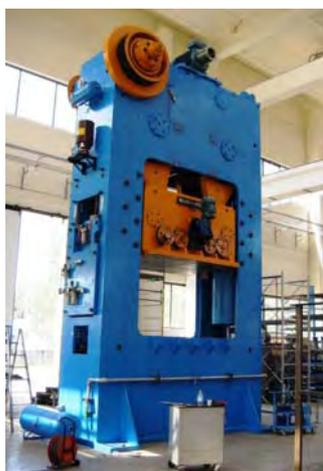
The overhauling and modernisation works of a large 15'000kN Wilkins & Mitchell mechanical trimming press are near to conclusion.
