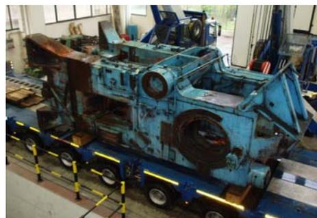
An important design modification was made by replacing the original brake with a new hydraulic brake system. An as NEW warranty is given on all rebuilt systems and rebuilding works. Over the past few years VALDARNO has rebuilt several large equipment from makers like Smeral, National, Farina and others, while overhauling works on a 4.000t Eumuco forging press are ongoing at present.
